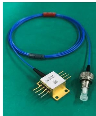
Figure 2.5 Compact III-V material based single photon detector
