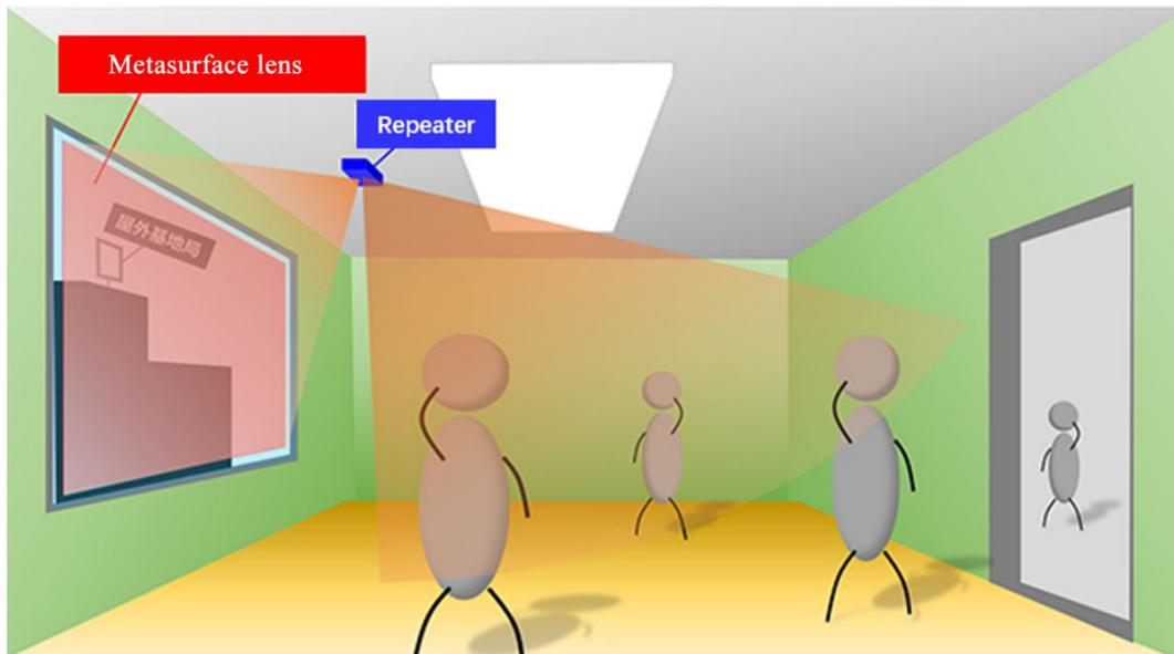
Figure 3-13 Metasurface Lens Combined with a Repeater installed on the Focus to Enhance Indoor Coverage [3]
