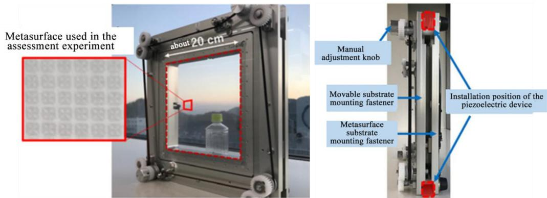
Figure 3-9 Appearance (Left) and Structure (Right) of a Millimeter-Wave Transparent Dynamic Metasurface[2]
