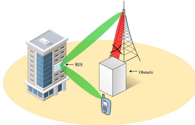
Figure 1-2 Coverage Hole Filling by RIS
