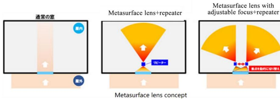
Figure 3-12 Common Glass, Fixed Metasurface Lens, and Dynamic Metasurface Lens (from Left to Right) [3]
