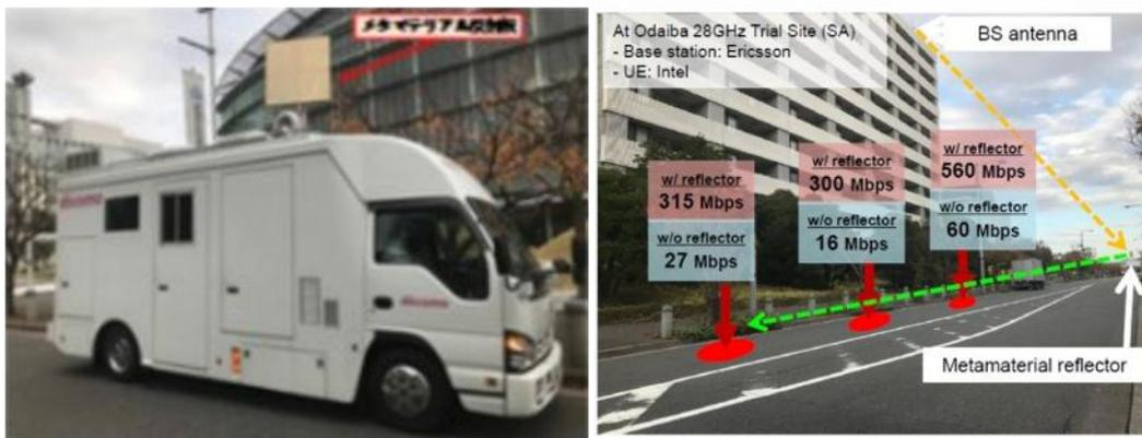
Figure 3-8 Onboard Millimeter-Wave Metamaterial Reflector (left); Test Scenario and Results (right) [1]
