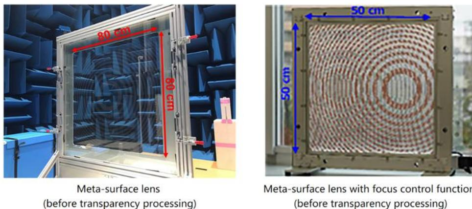
Figure 3-11 Fixed-Focus Metasurface Lens (Left) and Metasurface Lens with Focus Control Function (Right) [3]
