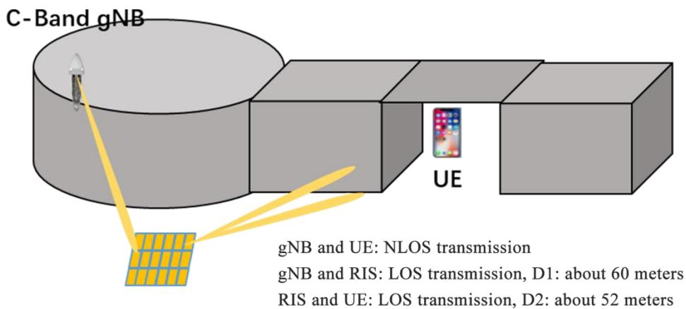
Figure 3-14 Deployment of the RIS Field Test Conducted by China Unicom and ZTE
