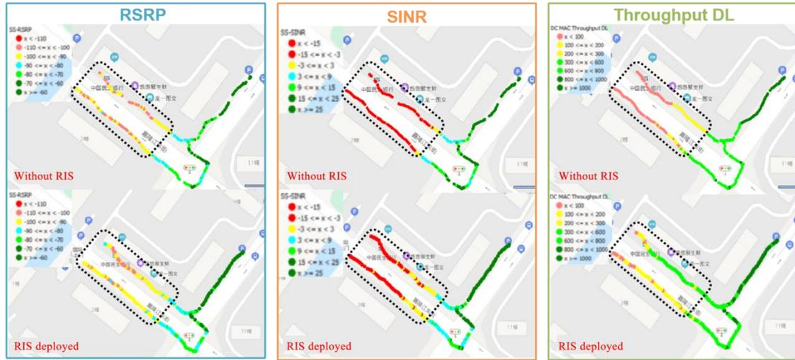
Figure 3-7 RSRP, SINR, Throughput Dot Figures in the Outdoor Traversing Test
