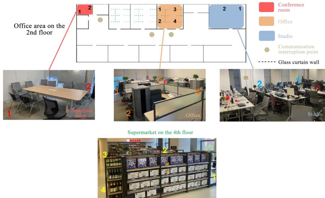
Figure 3-6 Schematic Plan for Fixed-Point Transmission Test in the Office Building
