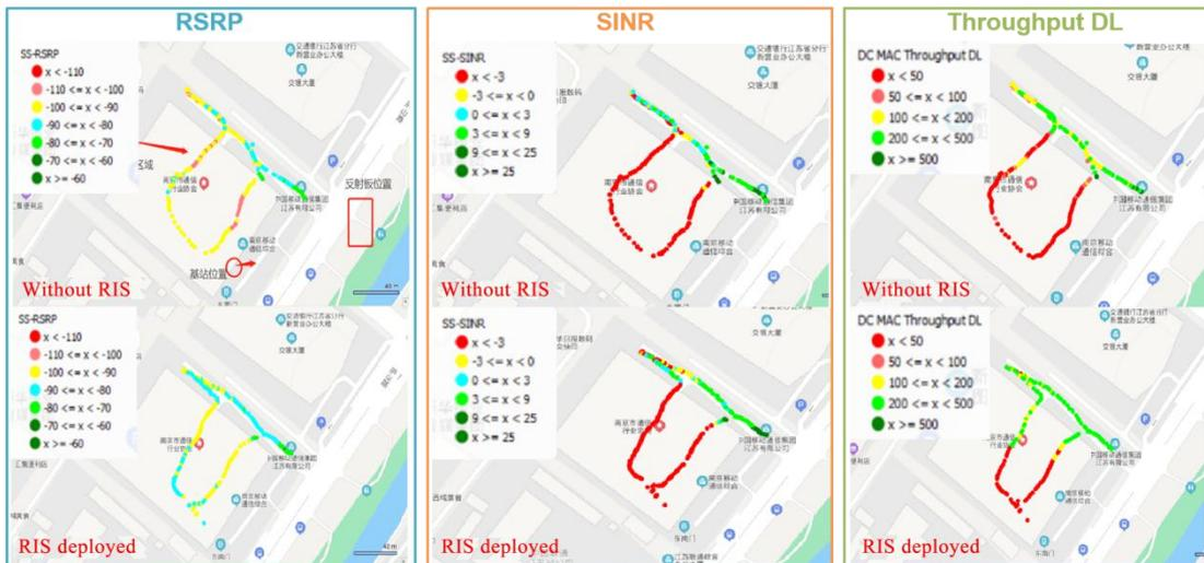
Figure 3-5 RSRP, SINR, Throughput Dot Figures Before and After RIS Deployment in Under-Tower Shadow Zone Test Case
