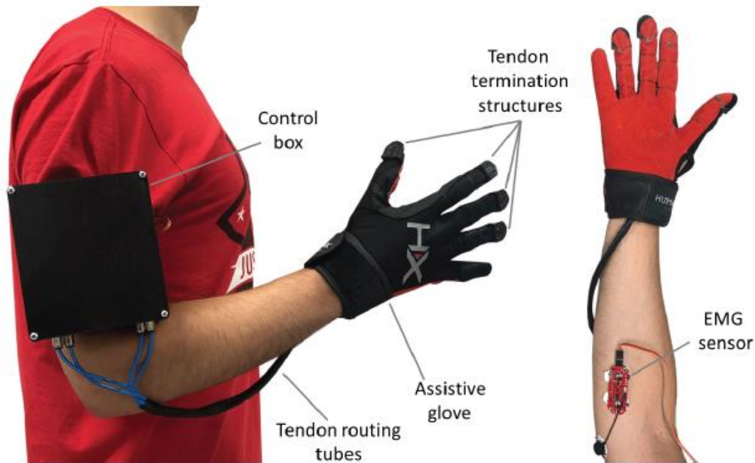
Fig. 1. The underactuated, tendon-driven, assistive exo-glove is composed of a control box, a glove, and an EMG sensor. The control box contains the motor that is connected to the proposed four-output differential mechanism. The differential is connected to four artificial tendons which are routed through tubes to reach the soft exo-glove. The tendons are connected to tendon termination structures stitched onto the fingertips of the exo-glove. The system is controlled by an EMG sensor located at the forearm.
