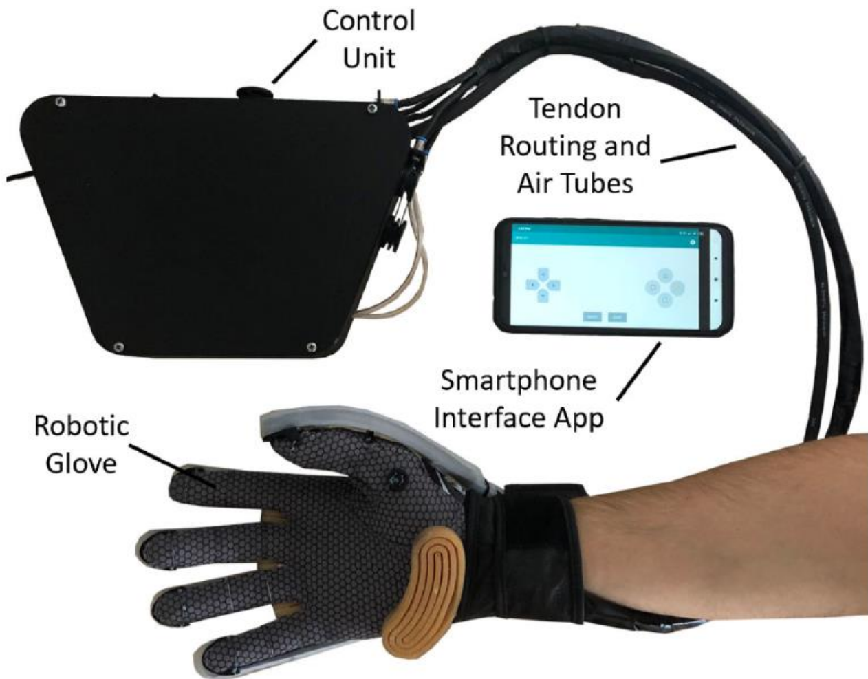
FIGURE 1. The hybrid exoskeleton glove is equipped with a tendon-driven system for finger flexion, pneumatic actuators for finger abduction, and an inflatable, telescopic extra thumb for grasp quality enhancement. The soft glove is connected to the control box that houses the actuators.
