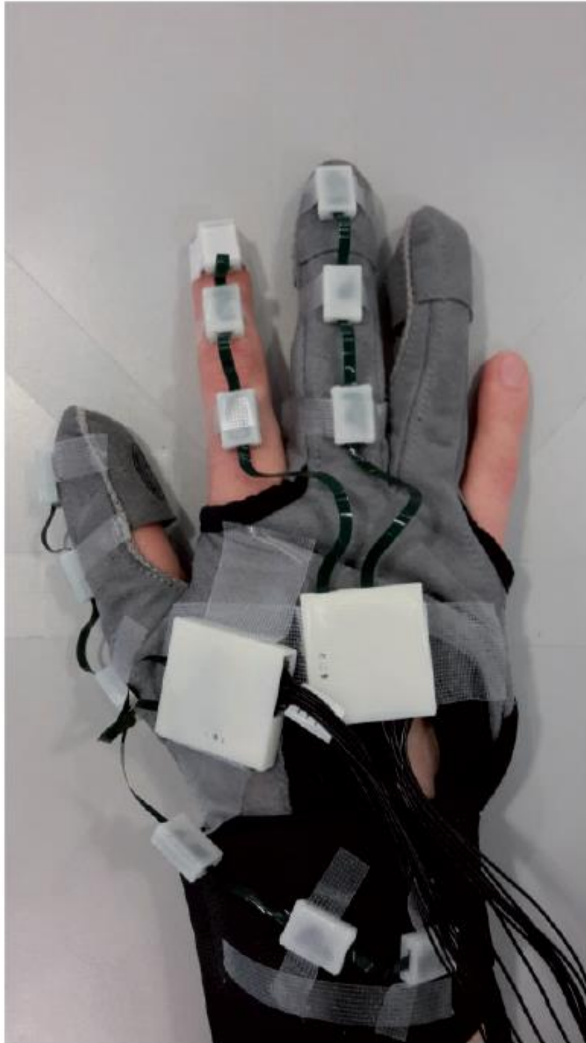
Figure 1. Instrumentation of the experiment. The SEM™ Glove is the soft-robotic glove worn by the subject. The white sensors are the IMUs.
