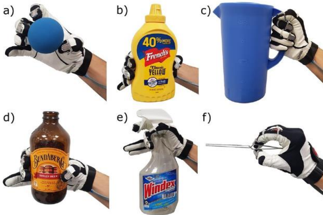
Fig. 8. Both devices were tested for grasping different types of objects: a) a ball, b) a mustard bottle, c) a jar, d) a glass bottle, e) a spray bottle, and f) tweezers.
