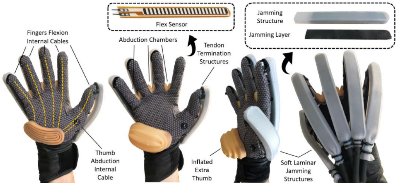
FIGURE 3. The soft glove system of the device consists of a glove, a tendon-driven system, and a pneumatic system that is composed of four soft actuators and five laminar jamming structures. Five plastic tendon termination structures are stitched onto the fingertip regions of the glove. The tendon-driven system has a tendon connected to each of the tendon termination structures and an extra tendon that is connected to the thumb's interphalangeal joint region, facilitating the execution of the opposition motion. The soft structures are used for three different purposes: to perform abduction/adduction of the fingers, to increase grasp stability by implementing an extra thumb structure, and to change the bending profile of the fingers. Three of the pneumatic chambers are connected to the region in between the fingers allowing for the execution of the abduction/adduction motion of the fingers. Another soft actuator was designed to act as a telescopic extra thumb that participates in grasping tasks, increasing the area of the contact patches between the hand and the object and increasing both grasp efficiency and stability. At the back of the glove, five laminar jamming structures were added to adjust the stiffness of the joints and to perform a locking motion to keep the hand in its natural, zero effort position. A flex sensor is located at the index finger and can be used to control the motion of the exoskeleton glove.
