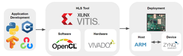
Fig. 8. Example of FPGA implementation flow using HLS tools presented in [36].
